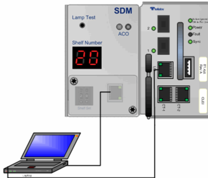
Figure 3.4 Cable Connections on the SDM and STPM
