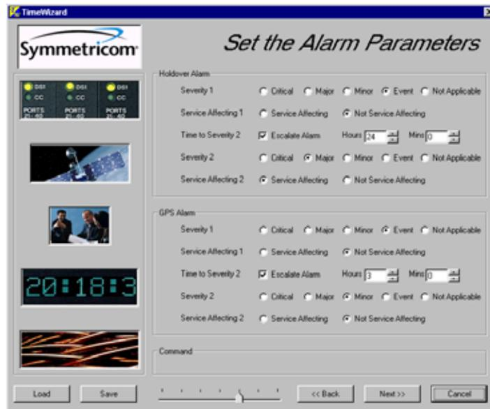
The Load and Save buttons allow a file to be generated that saves the alarm parameters in a file called TS3Kconf.sym as default. The file name for a configuration can be saved by selecting the Save button and providing a file name. The Load button allows the user to load a saved file that will automatically configure the Alarm Parameters screen.
