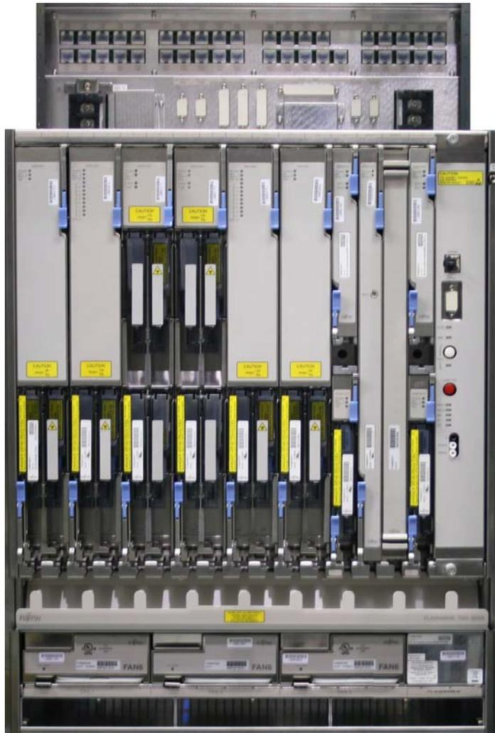
Figure 4-11: Optical Shelf—Populated with Plug-In Units (ETSI Configuration)
