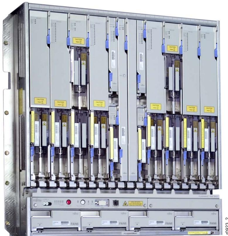
**Figure 2-13: Optical Shelf—Populated with Plug-In Units (Front View)
