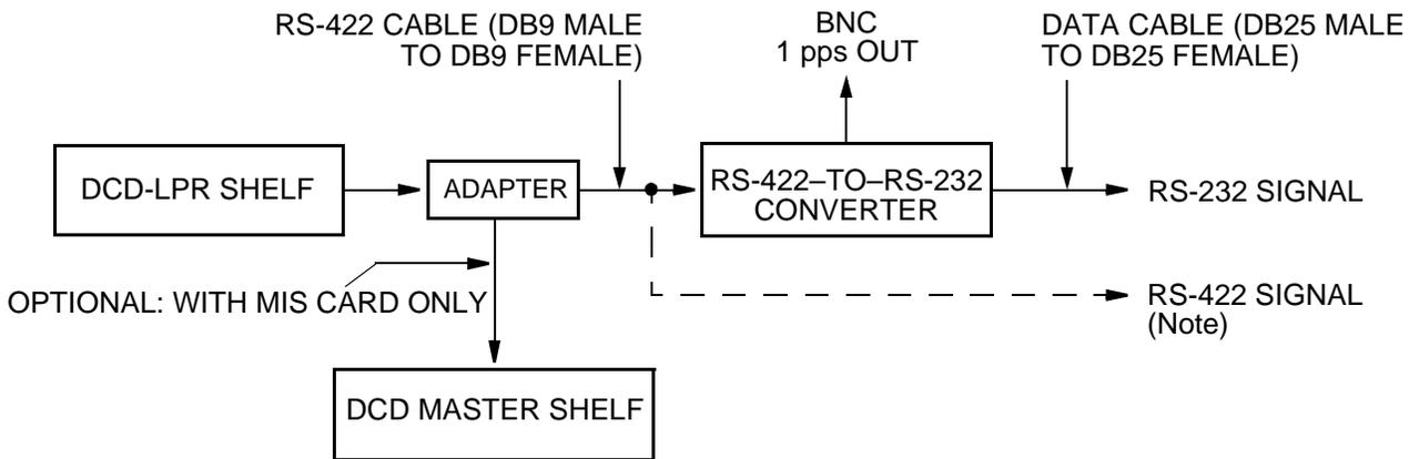
Note: RS-422-to-RS-232 converter not required for RS-422 signal.
