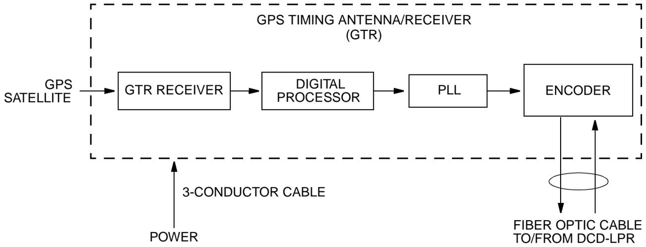
Figure 2. GTR Block Diagram
