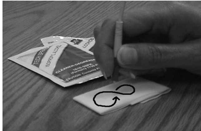
Figure B-1 Cleaning the Ferrule Endface
