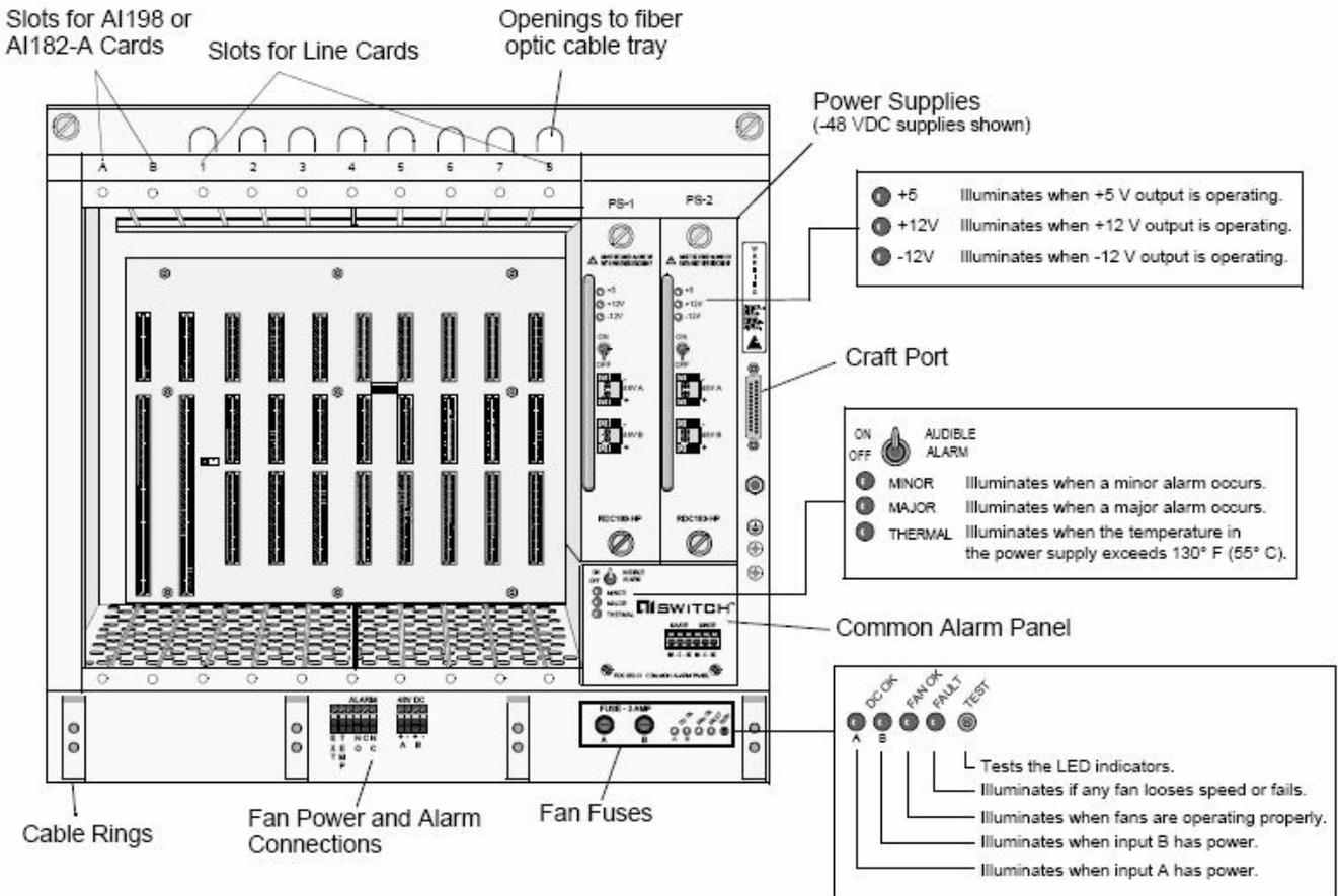
**CAUTION:** Personnel handling cards must wear an antistatic wrist strap and follow electrostatic procedures. For safety and proper cooling, cover all unused slots with a blank cover.
